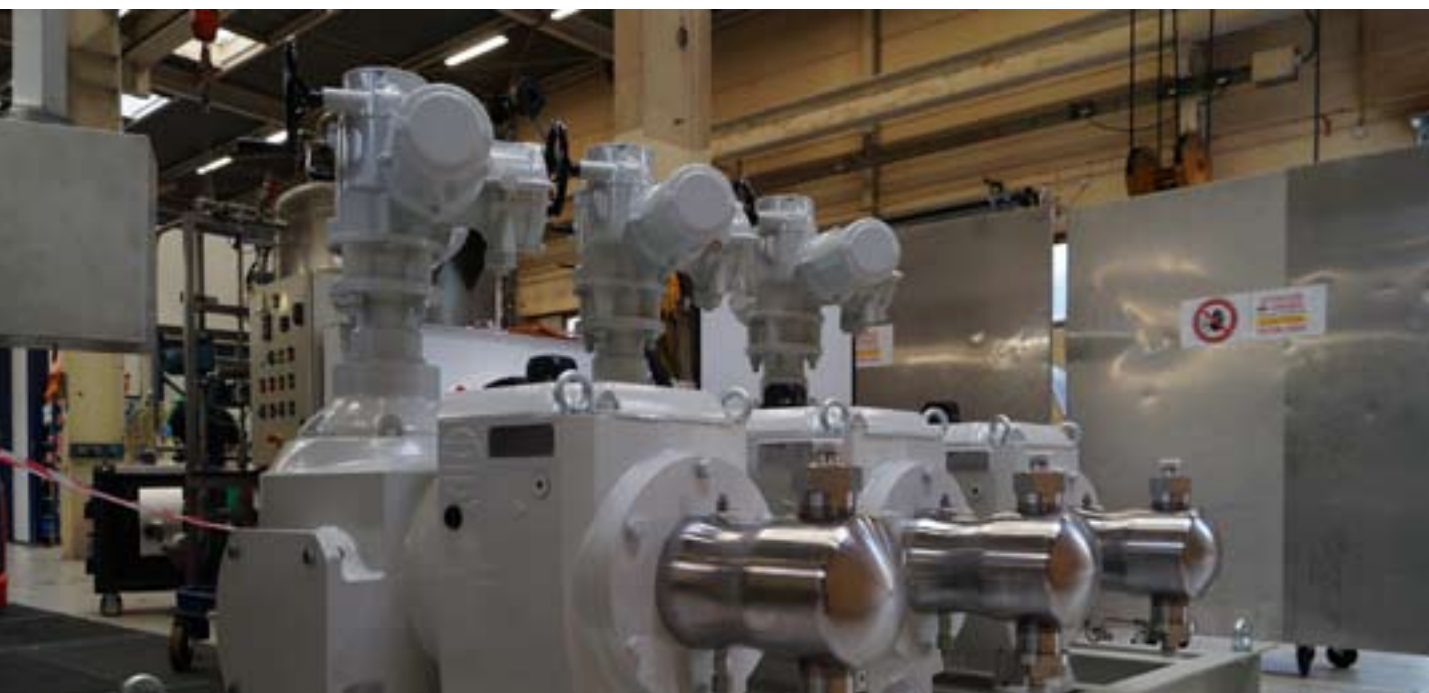
Milton Roy's Primeroyal R triplex metering pumps that were specially-configured to meet the project requirements.
